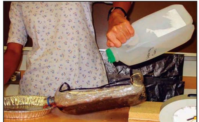
8) Immediately note the time in seconds when runoff starts to enter the empty pie pan. After sprinkling all two cups of water into the model students should observe the following using the data sheet as a guide: color of water and presence of oil, soil, and sprinkles in the pie pan.
